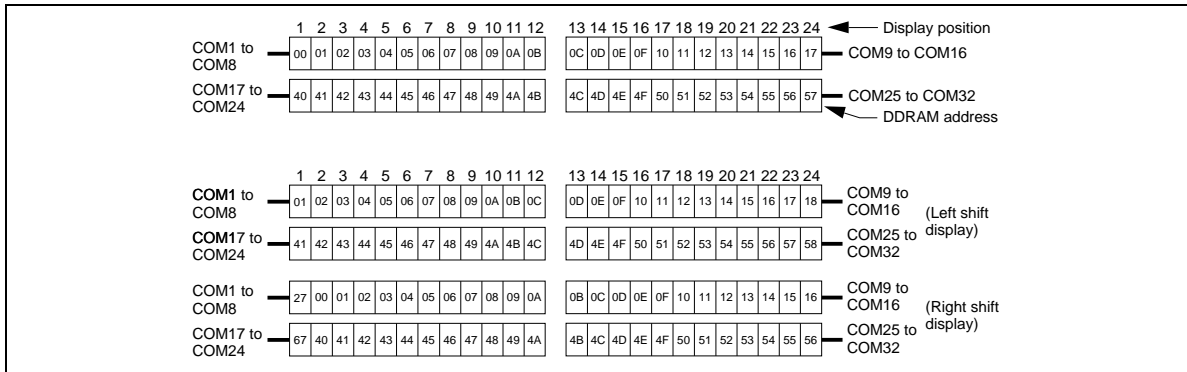
Figure 5 2-Line by 24-Character Display (5-Dot Font Width)
